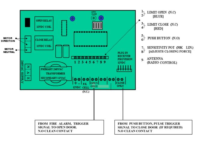
Fire alarm, when activated, will open door and as long as fire alarm signal is on the door will stay open via the "open only" input on Robot PCB. This signal will override any other triggering signal.
